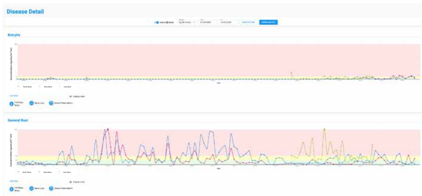
Figure 4. Example landing page for the regional disease surveillance network. Users can select multiple SporeScout units and view the spore concentrations of the pathogens we track. Users can filter the data by selecting specific SporeScout units and date ranges and can download the filtered data in a CSV file. Note: this is a mock-up and may vary from the real landing page.
